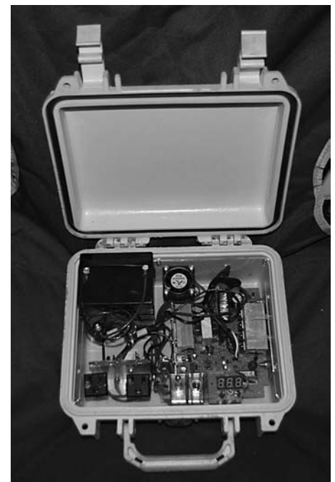
110-volt power supply in a Pelican Case
