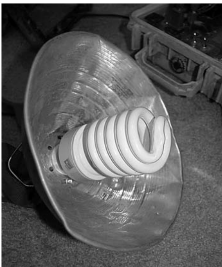
Compact fluorescent tube used for in-cave lighting of photographs
